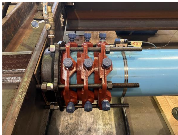
Figure 2-3 Attachment details on the reaction side.
