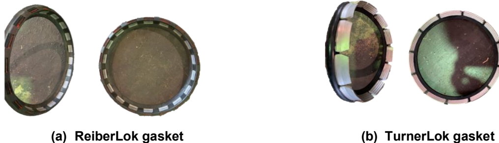
Figure 1-2 Gaskets for the specimens (a) for Specimen 1 (b) for Specimen 2
