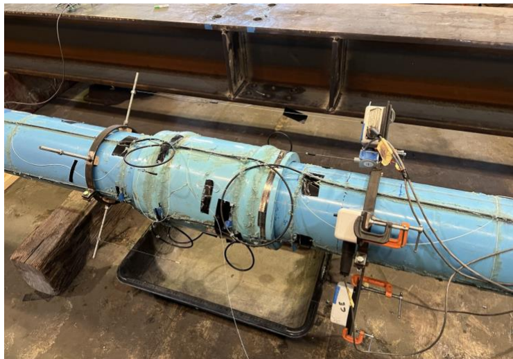
Figure 3-1 Position transducers for displacement monitoring of the joint.
