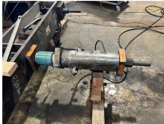
Figure 2-2 Hydraulic cylinder and load cell on loading side.
