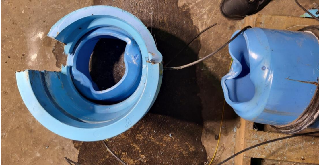
Figure 5-7 Severe material damage and local buckling at the beveled sides of both iPVC pipeline segments telescoping inside the coupling, following the compression test.
