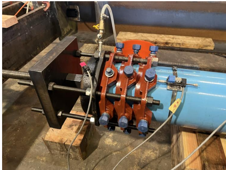
Figure 3-3 Transducer for monitoring the displacement of MegaLug
