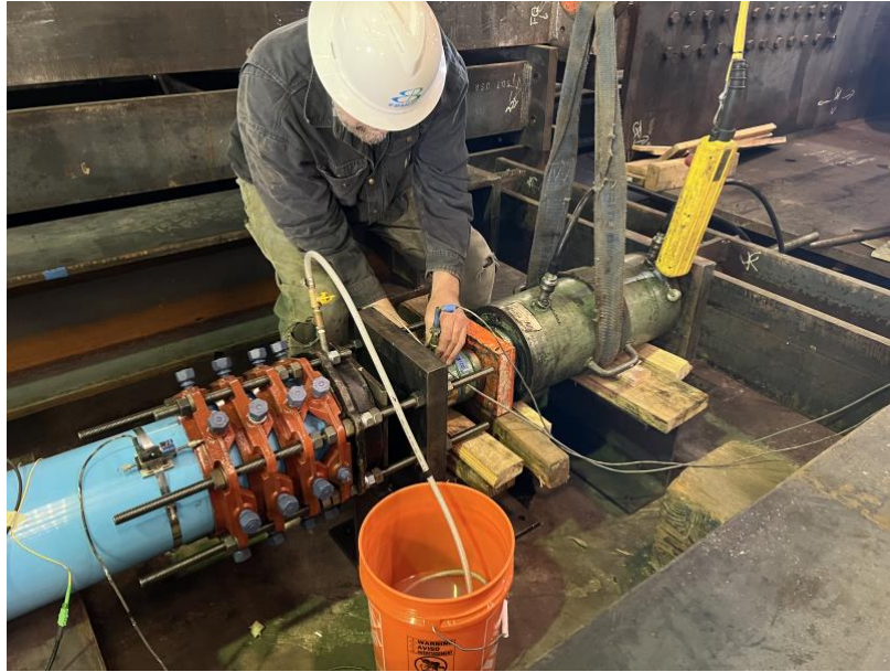
Figure 2-2 Hydraulic cylinder and load cell on the loading side
