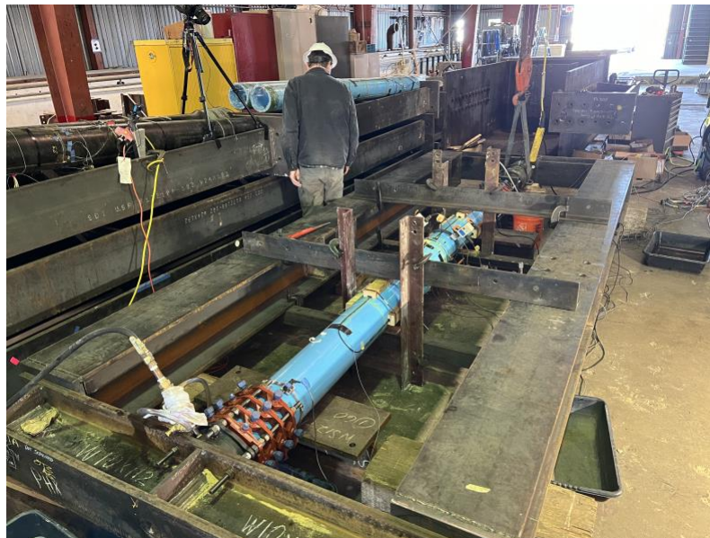
Figure 2-5 Photo of the completely assembled test setup: view from the reaction side
