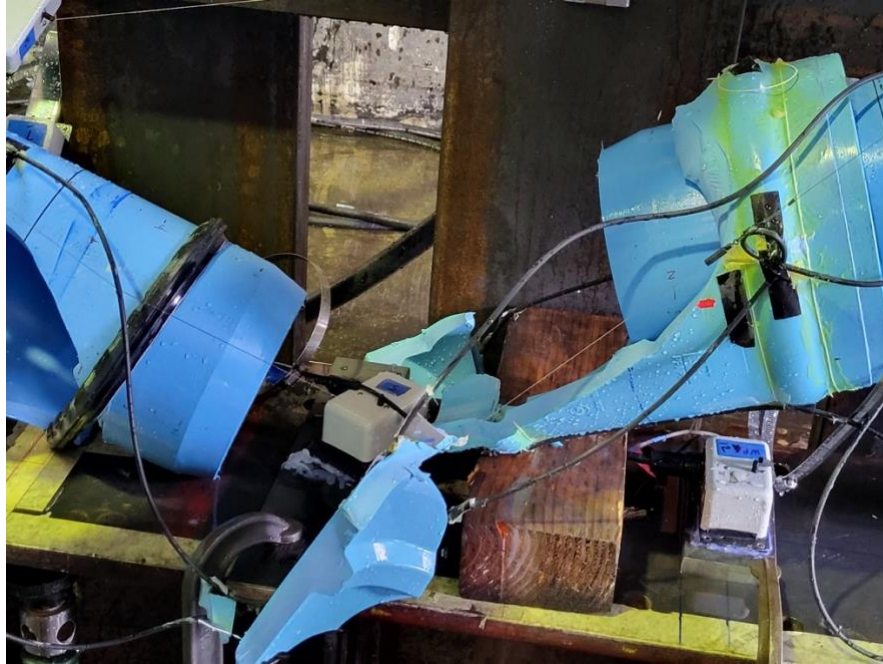
Figure 5-4 Failure of the jointed pipe system, originating at the top of the fitting and bottom of the left sided pipe at the gasket contact interface.
