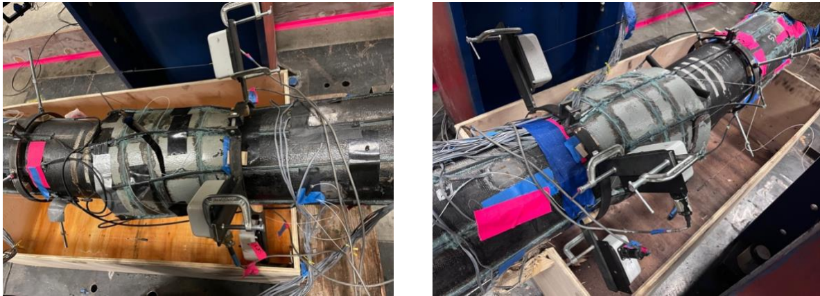
Figure 4-18 Failure of Bell of Specimen 1 (left) and 2 (right)
