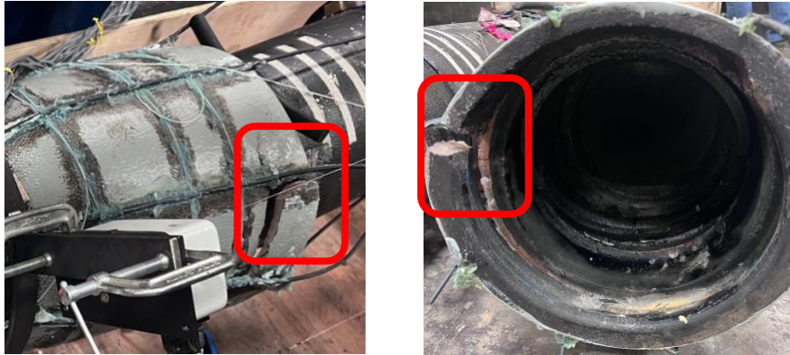
Figure 5-9 Failure mode – Specimen 2
