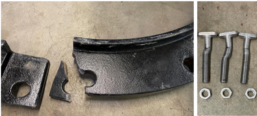
Figure 4-4 Failure of the gland and bolt
