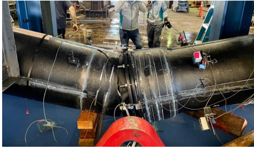
Figure 4-3 Large deformation and failure
