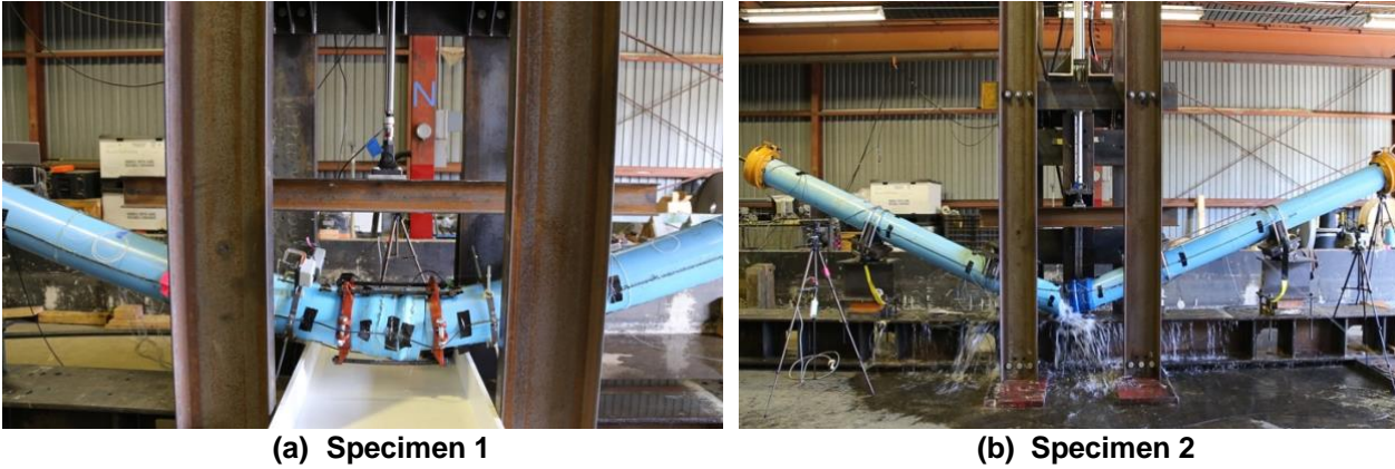
Figure 4-2 Large deformation of Specimen 1 and 2
