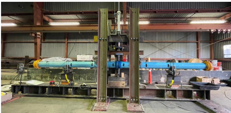
Figure 2-2 Specimen 2 (RCT restraint) experimental setup
