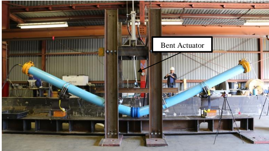
Figure A-1 Experimental setup and large deformation of the additional trial specimen
