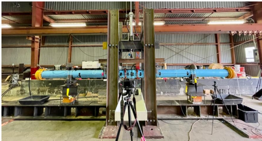
Figure 2-1 Specimen 1 (EBAA 1900 restraint) experimental setup
