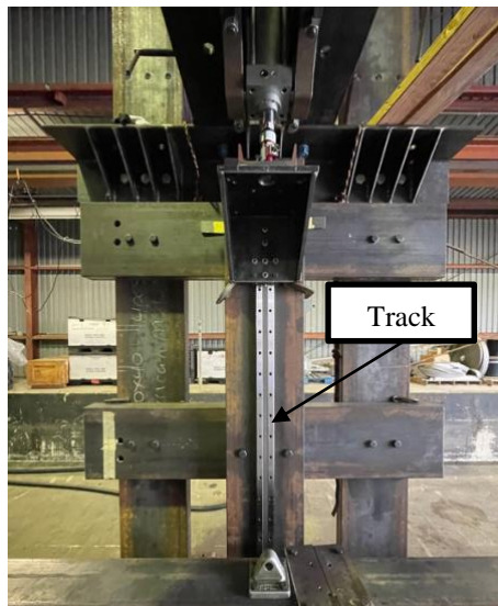
Figure A-2 Specially designed track for actuator
