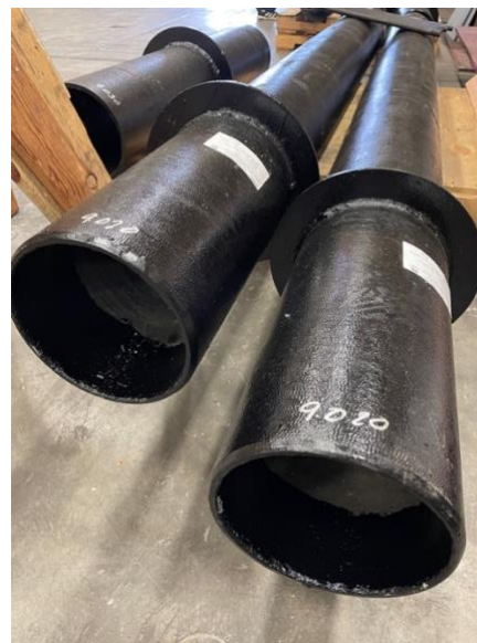
(b) Reinforced end weld bead for Specimen 2
