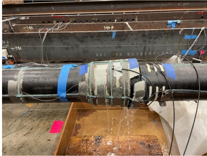
Figure 4-12 Failure of Bell of Specimen 2
