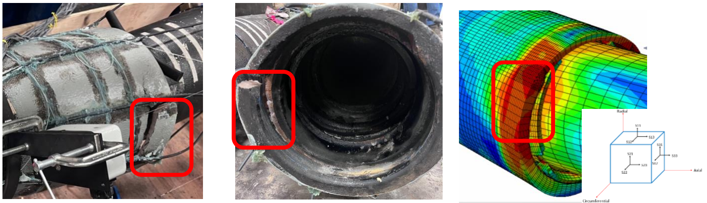
Figure 5-22 Failure mode comparison of Test 2
