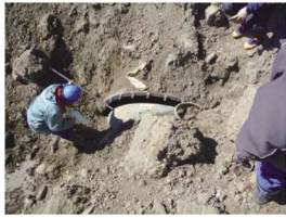
Fig. 26 五本松第1分水工周辺の片蓄管の離脱 Separation of a reducer around Gohomatsu No.1 division works
