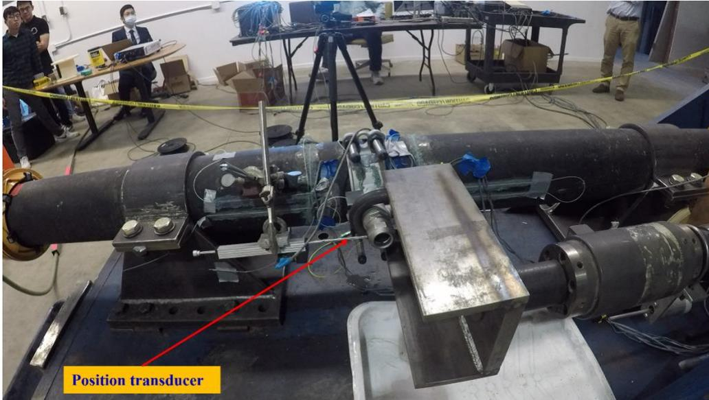
**Figure 3-2. Additional position transducer at saddle**
