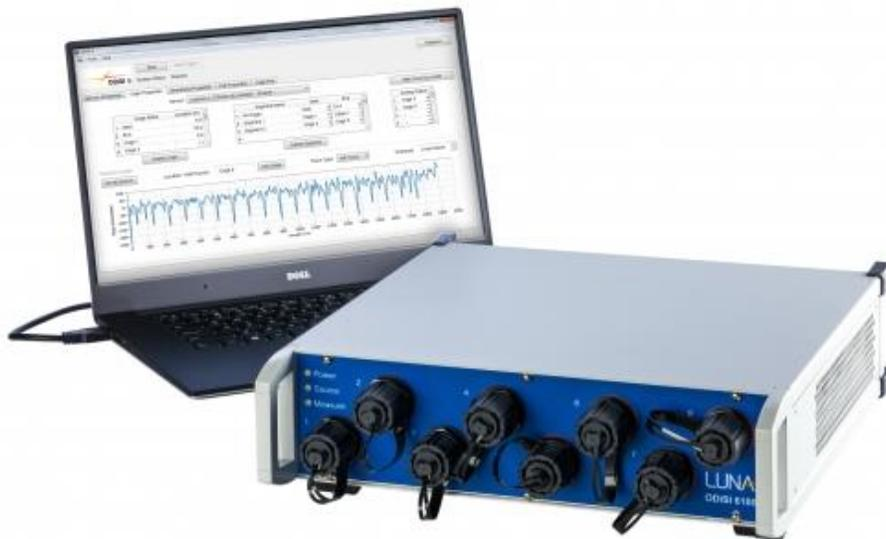
**Figure C-1. LUNA ODiSI 6000 Series optical distributed sensor interrogator**
