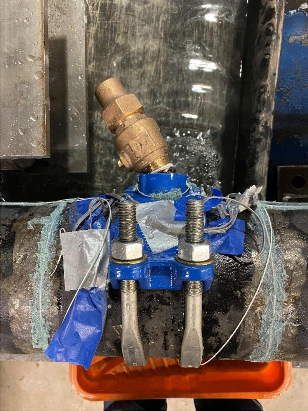
Figure B-1. Failure mode of benchmark saddle
