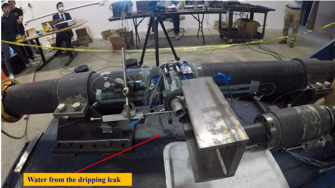
Figure 4-6. PowerSeal saddle: dripping water leak close to the maximum force
