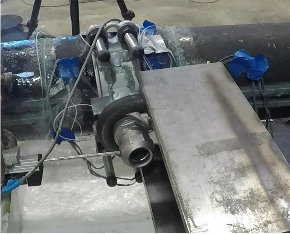
**Figure B-4. Side view of PowerSeal saddle: at completion of a test (typical)**
