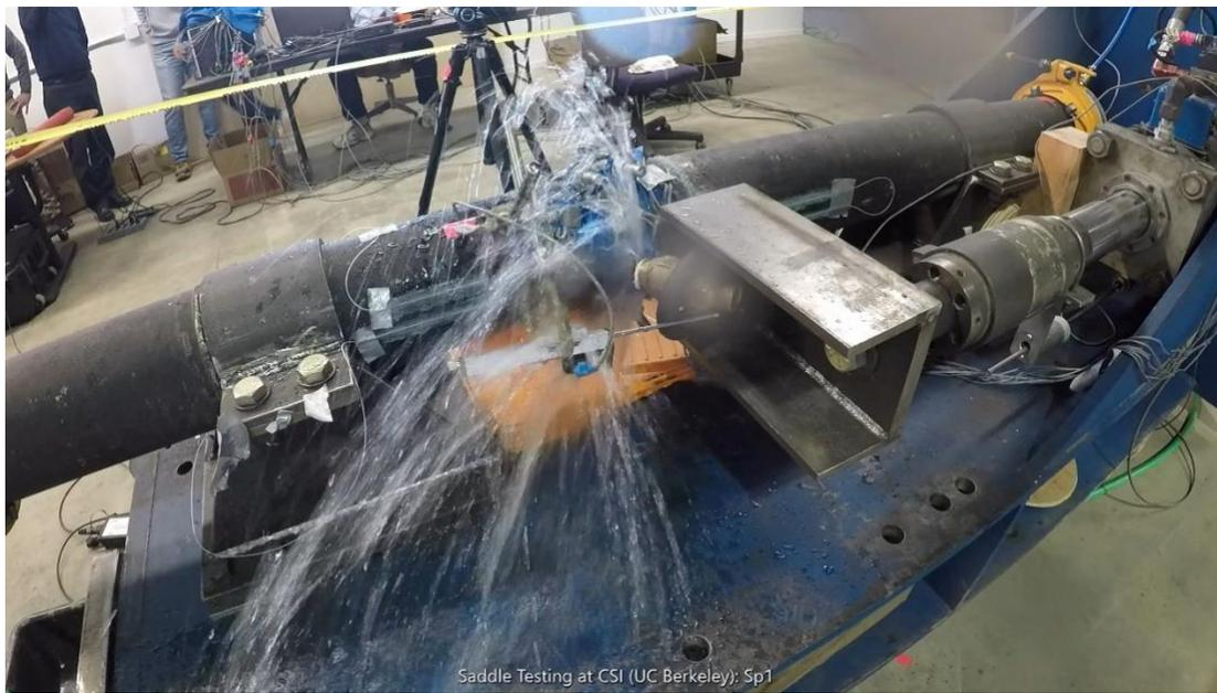
Figure 4-5. Typical failure of benchmark saddle
