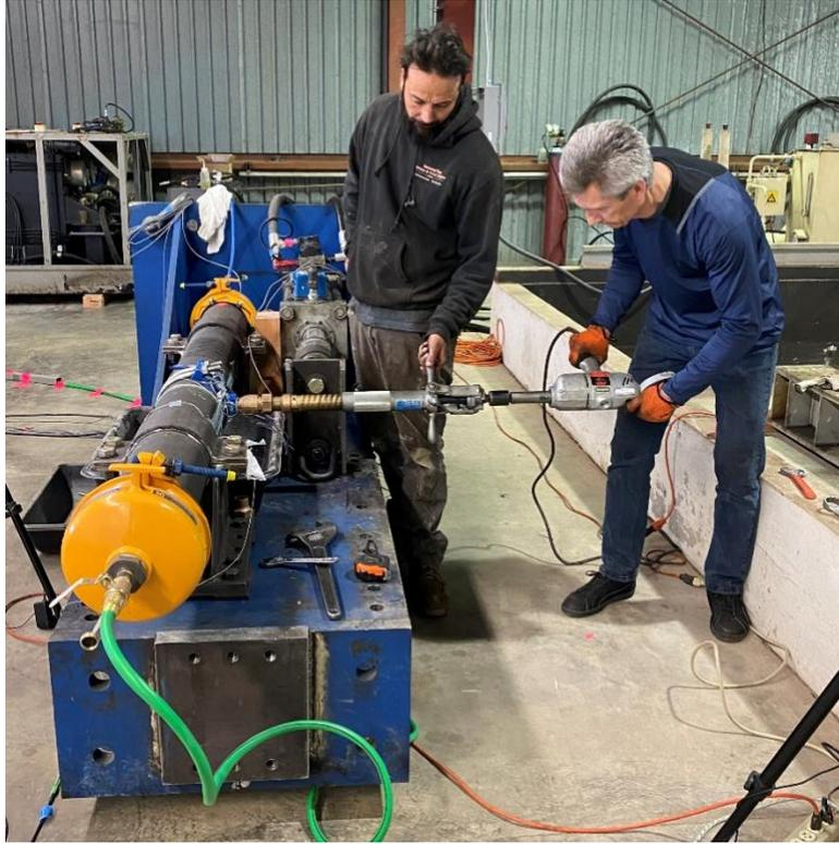
**Figure 2-2. Drilling a tap hole in distribution pipeline through a saddle**
